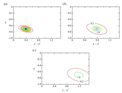
Figure 9. Contour plots of  $\kappa_{NLyy}(x-x',y,y',\tau)$  for turbulent channel flow obtained from the model in the x-y plane for y'=-0.7 at (a)  $\tau=0.025$ , (b)  $\tau=0.05$  and (c)  $\tau=0.075$ . The contour values range from 0.2 with an increment of 1.6.
