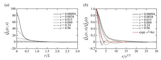
Figure 4. Profiles of two-point correlations at six scales in the scale space: (a)  $\hat{Q}_{ii}(r, s)$  as functions of r/L and (b)  $\hat{Q}_{ii}(r, s)/\hat{Q}_{ii}(s)$  as functions of  $r/s^{1/2}$ . The red line denotes the function  $\exp(-r^2/4s)$ .
