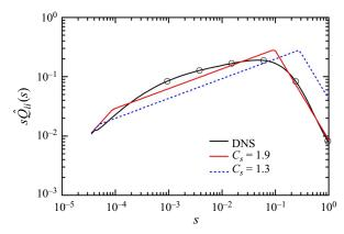
Figure 3. Profiles of the pre-multiplied energy density  $s\hat{Q}_{ii}(s)$  as functions of s for DNS and (3.20) with  $C_s = 1.3$  and 1.9. Symbols represent the locations of six scales at which two-point correlations are plotted in figure 4.
