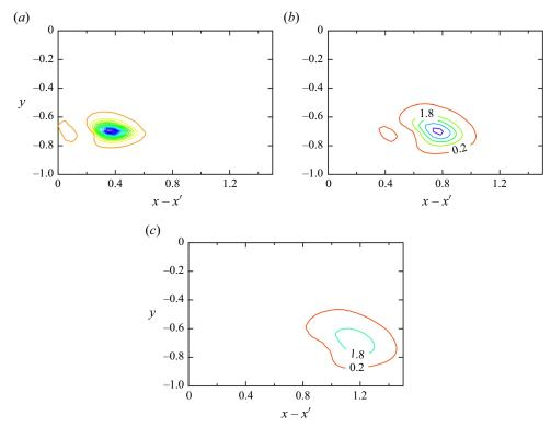
Figure 8. Contour plots of  $\kappa_{NLyy}(x-x',y,y',\tau)$  for turbulent channel flow obtained from the DNS in the x-y plane for y'=-0.7 at (a)  $\tau=0.025$ , (b)  $\tau=0.05$  and (c)  $\tau=0.075$ . The contour values range from 0.2 with an increment of 1.6.
