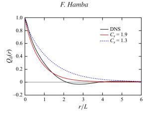
Figure 5. Profiles of two-point correlation  $Q_{ii}(r)$  as functions of r/L for DNS and the model given by (3.25) and (3.20) with  $C_s = 1.3$  and 1.9.
