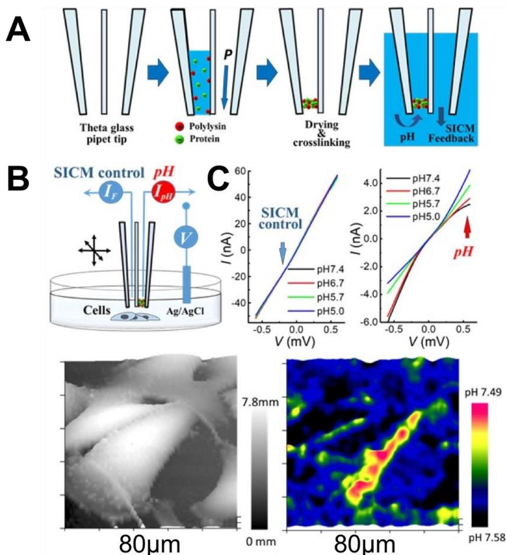
**Figure 1.** Fabrication of Scanning Ion Conductance Microscopy (SICM) feedback-controlled nanoprobe pH sensor to perform high-resolution 3D pHe mapping of living cells. (A) Cartoon of the fabrication
