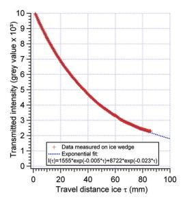
**Fig. 2.** Calibration curve (Eqn (1c)) derived from the measured transmission through a wedge of 86 mm side length made of pure bubble-free ice. The intensities are given in arbitrary grey-value units (a.u.). The curve fitting results in initial intensities  $i_{0\text{soft}} = 8722 \text{ a.u.}$  and  $i_{0\text{hard}} = 1555 \text{ a.u.}$  with attenuation coefficients  $k_{\text{soft}} = 0.023 \text{ mm}^{-1}$  and  $k_{\text{hard}} = 0.005 \text{ mm}^{-1}$ .
