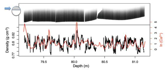
Fig. 6. Small-scale comparison of ln(Ca<sup>2+</sup>) and X2D density around the firn-ice transition along with an X2D scan (upper panel).
