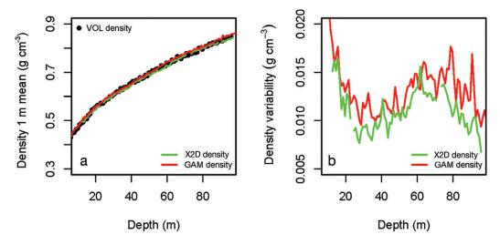
**Fig. 5.** Comparison of B32 mean density and density variability measured with different methods. (a) Bag mean density (1 m intervals) using the volumetric method (VOL), gamma-ray absorption (GAM) and the X2D technique. (b) Density variability (standard deviation over a 2 m running mean) using GAM and X2D density.
