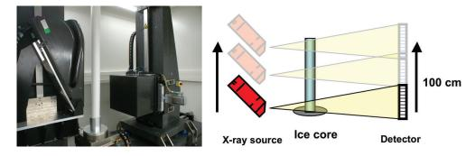
Fig. 1. Left: image of the ICE-CT inside the cold laboratory; right: a schematic view of the X2D scanning routine.
