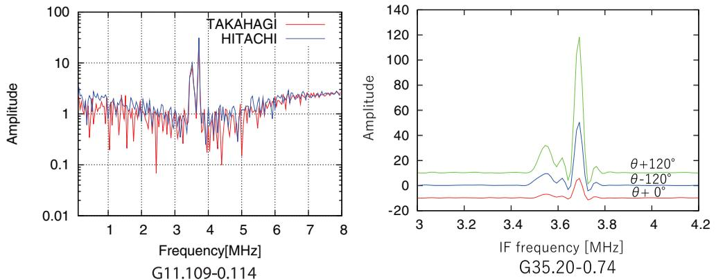
**Figure 2.** Left: Sample cross-spectra of the observed maser sources with Hitachi 32m and Takahagi 32m by the cross-correlation spectrometry. Right: The phase difference of two telescopes are obtained after comparing the XCS amplitudes of three cases of the phased result by adding an offset of  $120^\circ$ ,  $-120^\circ$ , and  $0^\circ$ . We added offsets to the plots for a clarity.
