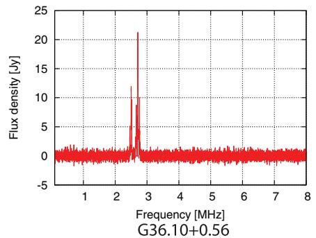
**Figure 1.** Sample Spectra of phased two telescope of Hitachi 32 m and Takahagi 32 m after digital position switching performed in 60 s integration and 1 kHz resolution.
