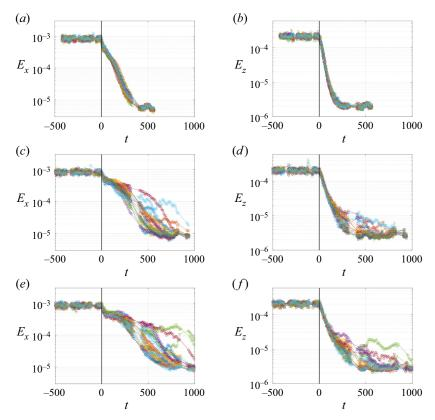
Figure 13. Temporal energy evolution of  $E_x$  (a,c,e) and  $E_z$  (b,d,f) for 20 quench experiment realisations at  $Re_f = 375$  (a,b),  $Re_f = 510$  (c,d),  $Re_f = 525$  (e,f); noise level: low ( $\sigma_C$ ).
