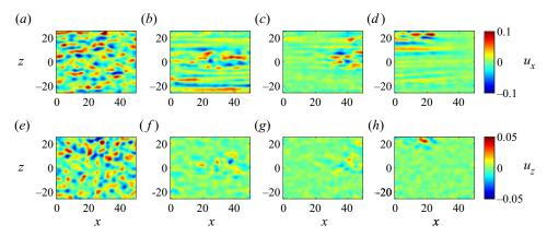
Figure 5. Snapshots of  $u_x$  (a–d) and  $u_z$  (e–g) at different times for  $Re_f = 600$ : (a,e) t = -215, (b,f) t = 430, (c,g) t = 1255, (d,h) t = 2430; noise intensity: high ( $\sigma = 4.6 \times 10^8$ , defined in § 4.1).
