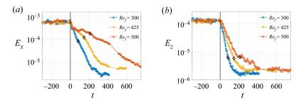
Figure 8. Temporal evolution of  $E_x$  (a) and  $E_z$  (b) for  $Re_f = 300$ , 425 and 500; black diamonds:  $\tau_z$  for each  $Re_f$ ; noise intensity: high ( $\sigma = 4.6 \times 10^8$ , defined in § 4.1).
