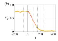
Figure 4. Temporal evolution of  $F_x$  (a) and  $F_z$  (b) for  $Re_f = 425$ ; dashed vertical lines represent the times for the snapshots of  $u_x$  and  $u_z$  plotted in figure 2; magenta dashed lines: linear fits  $F_i = a_i t + b$ , (i = x, z); black diamond: the position of  $\tau_z$  when  $E_z$  decreases to 5% of its initial energy; noise intensity: high ( $\sigma = 4.6 \times 10^8$ , defined in § 4.1).
