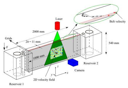
Figure 1. A schematic diagram of the experiment.
