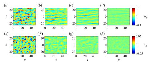
Figure 2. Snapshots of velocity fields for different times at  $Re_f = 425$ . (a-d) Velocity fields in the streamwise direction  $u_x$ , (e-h) velocity fields in the spanwise direction  $u_z$ . Times: (a,e) t = -65 (fully turbulent flow,  $Re_i = 1000$ ), (b,f) t = 91, (c,g) t = 150, (d,h) t = 286; noise intensity: high  $(\sigma = 4.6 \times 10^8)$ , defined in § 4.1).
