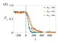
Figure 9. Temporal evolution of  $F_x$  (a) and  $F_z$  (b) for  $Re_f = 300$ , 425 and 500; black diamonds:  $\tau_z$  for each  $Re_f$ ; noise intensity: high ( $\sigma = 4.6 \times 10^8$ , defined in § 4.1).
