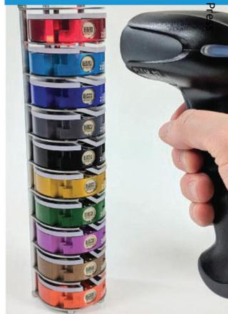
2D Barcoding and custom puck serialization for advanced sample tracking
