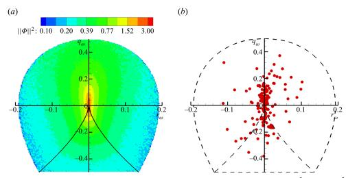
Figure 11. (a) Conditional average of the Frobenius norm of the vorticity gradient tensor  $(\langle \Phi^2 | r_\omega, q_\omega \rangle / \langle \Phi^2 \rangle)$  in the  $q_\omega - r_\omega$  plane for  $Re_\lambda = 225$ ; (b) scatter plot of extreme vorticity magnitude ( $\|\Phi\|^2 > 1000$ ) in the  $q_\omega - r_\omega$  plane.
