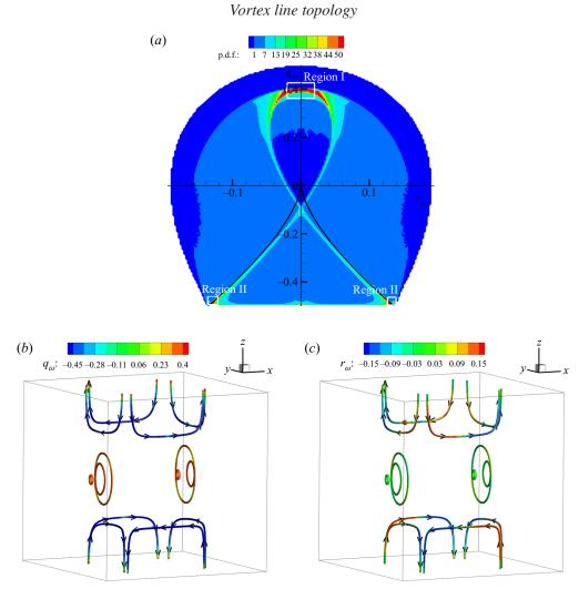
Figure 12. (a) Filled contour plot of the  $q_{\omega}$ - $r_{\omega}$  joint p.d.f. for the initial field of a Taylor-Green vortex flow. Field vortex lines in physical space dominated by regions I and II of the  $q_{\omega}$ - $r_{\omega}$  joint p.d.f. coloured by (b)  $q_{\omega}$  (c)  $r_{\omega}$ .
