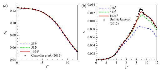
Figure 3. Time evolution of (a) normalized kinetic energy  $(E/U_0^2)$  and (b) normalized mean dissipation rate  $(\epsilon/(U_0^3/L))$  for a Taylor–Green vortex.
