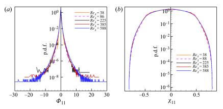
Figure 7. Marginal p.d.f. of the longitudinal component of the (a) un-normalized  $(\Phi_{11})$  and (b) normalized  $(\chi_{11})$  vorticity gradient tensor.
