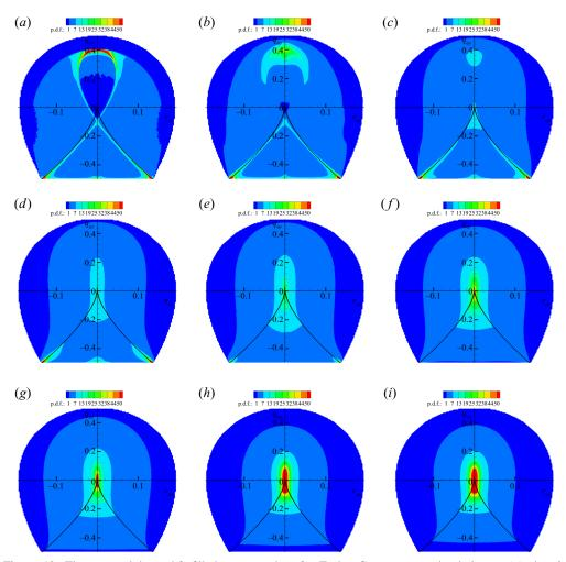
Figure 13. The  $q_{\omega}$ - $r_{\omega}$  joint p.d.f. filled contour plots for Taylor–Green vortex simulation at (a)  $t^*=0$ , (b)  $t^*=0.132$ , (c)  $t^*=0.145$ , (d)  $t^*=0.160$ , (e)  $t^*=0.185$ , (f)  $t^*=0.740$ , (g)  $t^*=5$ , (h)  $t^*=9.23$  and (i)  $t^*=11.57$ .
