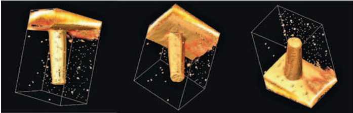
Fig. 27. Three different views of a vertical metal interconnect reconstructed from a tilt series using high angle annular darkfield Scanning Transmission Electron Microscopy (STEM)[5].
