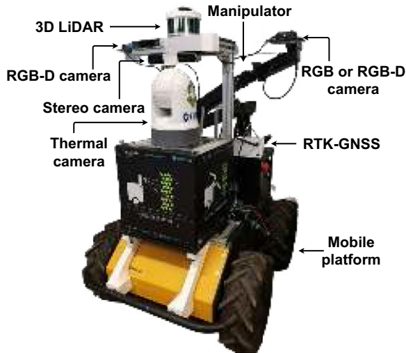
Figure 1. Robot AgRob v16 from INESC TEC to operate under open-field and controlled agricultural environments.
