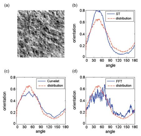
**Fig. 3.** (a) A simulated fiber network, (b) the result of a structure tensor -based orientation analysis of the network of figure (a), (c) the result of a curvelet-based orientation analysis of this network, and (d) the result of an FFT-based orientation analysis of this network. The known orientation distribution is shown by the dashed line for comparison.
