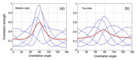
Fig. 9. Fiber-orientation distributions in a paper sample (top and bottom surface) for different orientations of the light source.
