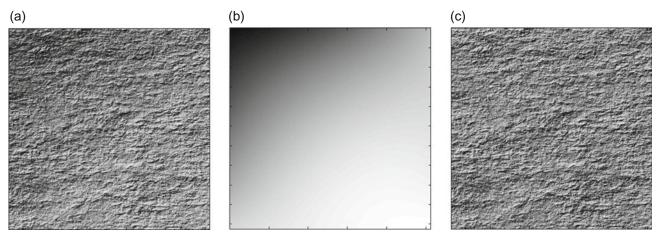
Fig. 2. (a) An original image of a paper sample. This image contains light reflected from the sample and effects of uneven illumination, (b) the estimated distribution of illumination and (c) the image resulting from removal of the estimated unevennes in the illumination.
