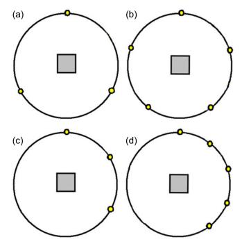
**Fig. 7.** A schematic layout of the illumination systems composed of three (a, c) and five (b, d) regularly spaced light sources.
