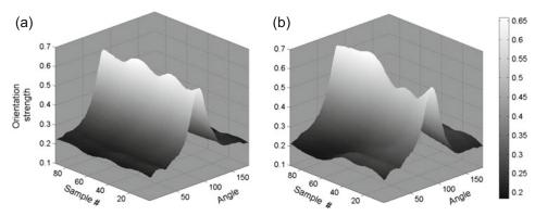
Fig. 12. (a) The average orientation distribution of the three-light illumination system shown in Figure 11d in a three-dimensional representation in which the orientation intensity appears as the third dimension (b) the three-dimensional orientation diagram (average) for a three-light system in which the intensity of one light source was decreased by 40%. The grey scale bar shows how the normalized orientation intensities are related to the grey scales.
