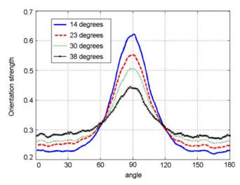
**Fig. 6.** Orientation distributions with three light sources placed at regular angular intervals for different inclination angles.
