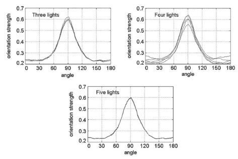
Fig. 8. Orientation distributions for illumination systems composed of three, four and five regularly spaced light sources at an inclination angle of  $14^{\circ}$ . For each system this distribution was determined every time the illumination system was rotated by about  $10^{\circ}$  from its previous position.
