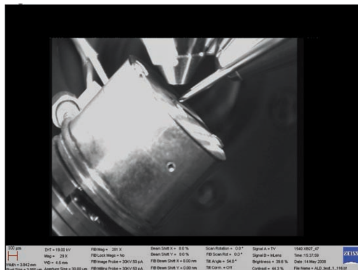
Figure 4: The single GIS nozzle extends from the right in the image and is directed through a circular opening on the lid of the heater substage. The heater substage acts as a gas concentrator for the GIS-ALD experiments.
