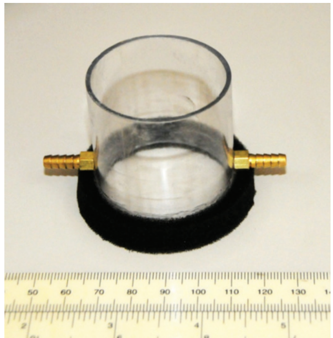
Figure 3: Chamber that seals the leaf from the atmosphere, shown here with the lower foam gasket that seals the leaf (sealing material for the objective lens is not shown).
