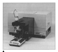
Fast Analytical Raman Spectroscopy System: The Explorer Series I from Instruments S.A. uses laser and filter technology, spectroscopic components, and data handling software to provide analysis results. The reduced-footprint system is suitable for R&D labs, production control labs, or contract analytical labs. Applications include chemicals and polymers, semiconductor materials, pharmaceuticals, and environmental monitoring.
