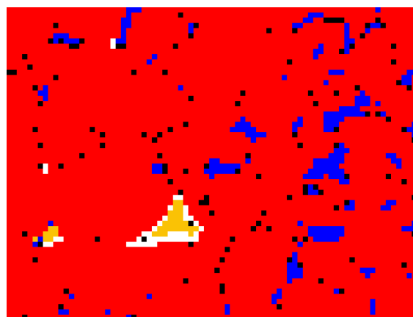
Figure 3. (above) K-means cluster analysis of the merged EDS and crystallographic information. Black: Matrix, unindexed. Red, TiB 2 hexagonal. Blue: Ti(CNO), cubic. White: (Ti,Zr,Al) oxide, cubic, with strong B signal. Yellow: (Ti,Zr,Al) oxide, cubic, weak B signal.
