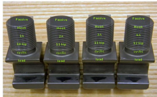
Fig 4. Post test photographs of the passive hook test articles.
