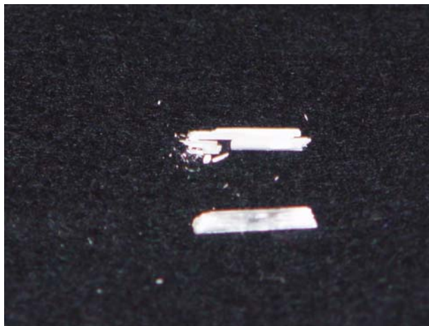
FIG 2. Photograph of kernite before (intact, bottom) and after (crumbling, top) vacuum dehydration.
