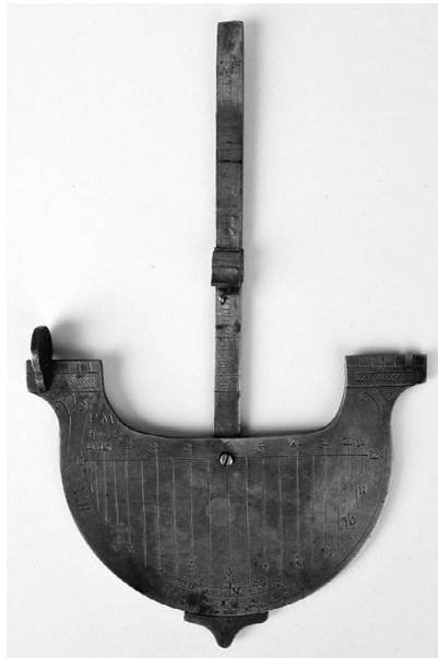
Figure 2.1 A navicula sundial in the Whipple Museum's collection, made in the eighteenth or nineteenth century, closely following the diagrams in medieval manuscript texts. Image © Whipple Museum (Wh.5902).
