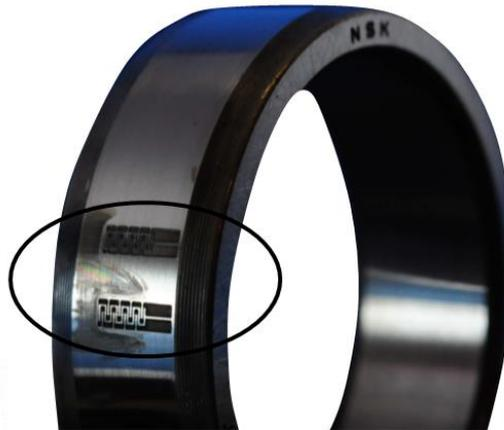
Figure 2: Rolling bearings with sensors to measure the elongation of the bearing rings (Winkelmann, 2014)
