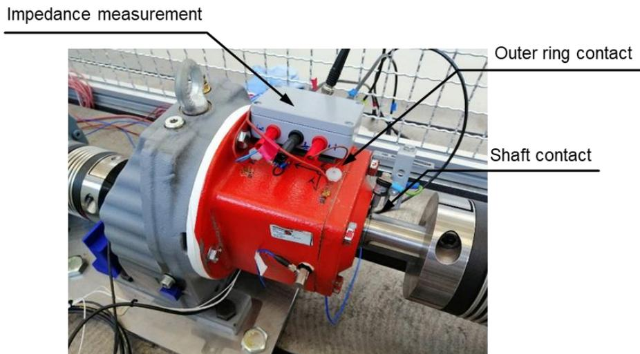
Figure 8: Prototype of the sensor rolling bearing in the industrial gearbox
