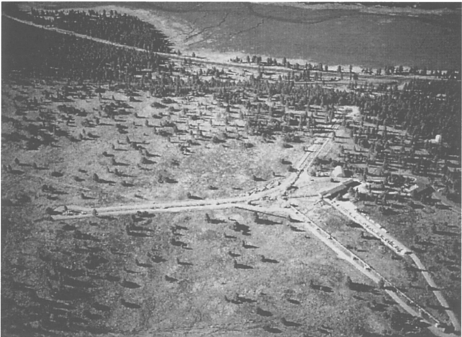
Figure 1. Aerial view of the Navy Prototype Optical Interferometer on Anderson Mesa near Flagstaff, Arizona. The north arm of the array extends from the center to the lower right corner of the picture. The four astrometric huts are at the center of the array. The pipes along the arms are for the vacuum feed system which brings light from the siderostats to the optics laboratory, which is the long building to the right of the array center.
