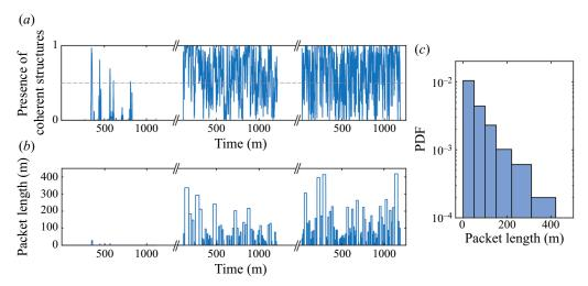
Figure 5. (a) The level of coherent structures from image classification, with a dashed grey line indicating the threshold, used to determine (b) the coherent structure packet length scale. (c) The PDF of the packet length for all three datasets. Note that the bin size is gradually increased for events with larger packet lengths to ensure sufficient statistical convergence for events with lower probability of occurrence.
