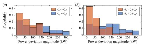
**Figure 13.** Magnitude of power deviation magnitude conditionally sampled by vortex size, including (a) a comparison between the vortices below and above the mean value of vortex size  $(\langle d_{eq} \rangle)$ , and (b) a comparison between vortices in the bottom and top quartile of vortex size  $(Q_1(d_{eq}))$  and  $Q_3(d_{eq})$ , respectively).
