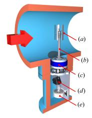
**Figure 2.** Rendering of VAWT model in a cutaway of the HRTF test section. Labels correspond to (a) 5-bladed VAWT model, (b) tower housing, (c) six-component force/moment sensor, (d) torque transducer with speed encoder and (e) magnetic hysteresis brake for speed control. Flow direction is given by the red arrow.
