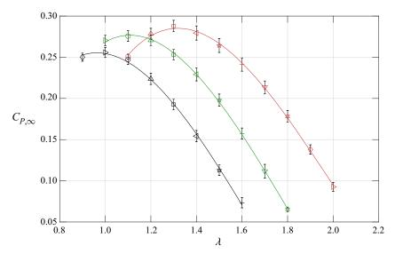
*Figure 7.* Reynolds invariant power coefficient as a function of tip speed ratio for varying solidity. Colour indicates solidity/blade number:  $\sigma_s = 0.36$  are black;  $\sigma_s = 0.29$  are green;  $\sigma_s = 0.21$  are red.
