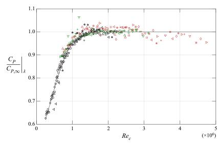
**Figure 8.** Power coefficient normalized by the Reynolds invariant value for three different VAWT rotor solidities. Symbol indicates  $\lambda$ , as in figures 5 and 7. Colour indicates solidity:  $\sigma = 0.36$  are black;  $\sigma = 0.29$  are green;  $\sigma = 0.21$  are red. The grey line is the curve fit from (3.4).
