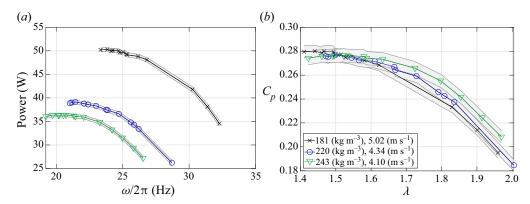
**Figure 6.** Dimensional power and rotation rate for the 2-blade turbine are shown for various tunnel conditions in panel (a) at a fixed Reynolds number of  $Re_D = 3.938 \times 10^6 \pm 4.1 \times 10^3$ . The data are then non-dimensionalized and plotted in panel (b) to illustrate data collapse due to dynamic similarity. The grey bars indicate measurement uncertainty of the data. The legend applies to both plots.
