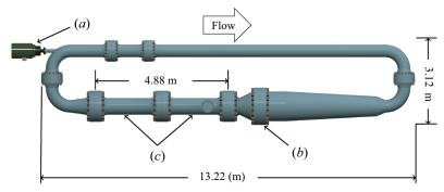
*Figure 1.* Schematic diagram of the HRTF as viewed from above the facility. The figure labels correspond to: the 150 kW pump motor (a), the flow conditioning and contraction (b), and the two test sections (c).
