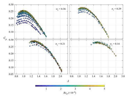
Figure 4. Power coefficient as a function of tip speed ratio for four different VAWT rotor solidities. Colour gives the mean  $Re_D$  value for each power curve. Two additional, high-Reynolds-number runs are available for the  $\sigma_s = 0.21$  rotor at  $Re_D = 5.93 \times 10^6$  for the grey-filled square symbols and at  $Re_D = 7.19 \times 10^6$  for the red-filled diamond symbols. Solid lines are cubic polynomial fits to the data.
