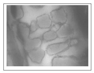
Fig. 4. Treated 15705 hours at 950 °C
