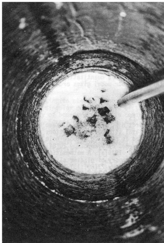
Fig.1. Photograph of bed and bottom of bore hole on Agassiz ice cap, northern Ellesmere Island, at 337 m depth. Darker vertical lines on top left- and lower right-hand sides of photograph are due to melting by heated melt tubes in thermal drill.
