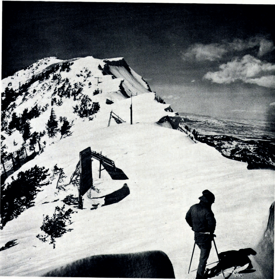
Fig. 1. View northward along Bridger Ridge showing cornice research area, Bridger Range, Montana. Structures are used for cornice control by redirecting wind.
