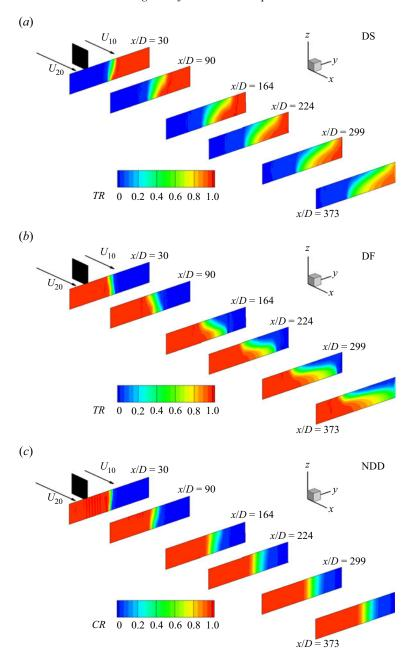
Figure 2. Non-dimensional density/temperature, TR, and passive scalar, CR, at several cross-sections in the mean flow. (a) Case DS; (b) case DF; (c) case NDD. The aspect ratio is x:y:z=10:10:1. For cases DS and DF, TR=1 and TR=0 are the non-dimensional densities of the incoming streams containing heavier and lighter fluid, respectively. For case NDD, CR=1 and CR=0 are the non-dimensional scalar concentrations of the incoming streams.
