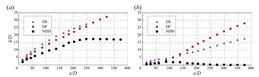
Figure 5. Mixing layer width as a function of the distance from the origin. (a)  $\delta/D$ ; (b)  $\delta'/D$ . The two variables are defined in figure 1.
