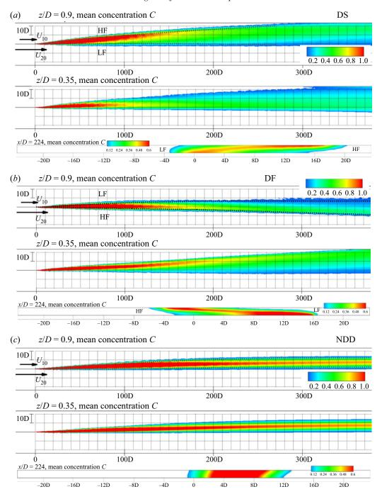
Figure 4. Non-dimensional scalar concentration, C, in the mean flow in the z/D = 0.9, z/D = 0.35 and z/D = 224 sections. C = 100 is used for the concentration at the end of the splitter plate to visualize the structure of the MI. (a) Case DS; (b) case DF; (c) case NDD. HF and LF denote the regions containing heavier and lighter fluid, respectively. Regions with C < 0.09 were blanked. The dashed lines show the boundaries of the MI in the z/D = 0.9 plane.
