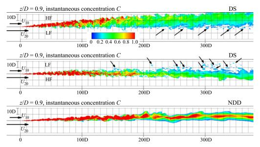
Figure 6. Non-dimensional scalar concentration, C, in the instantaneous flow near the free surface (z/D=0.9). C=100 is used for the concentration at the end of the splitter plate to visualize the structure of the MI. Regions with C<0.09 were blanked. HF and LF denote the regions containing heavier and lighter fluid, respectively. The black arrows point toward isolated spots of MI fluid reaching the free surface.
