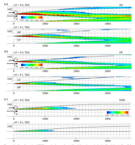
Figure 11. Non-dimensional TKE near the free surface (z/D = 0.9) and near the bed (z/D = 0.1). (a) Case DS; (b) case DF; (c) case NDD. HF and LF denote the regions containing heavier and lighter fluid, respectively. Regions with TKE < 0.004 were blanked. The dashed lines show the boundaries of the MI in each horizontal plane.
