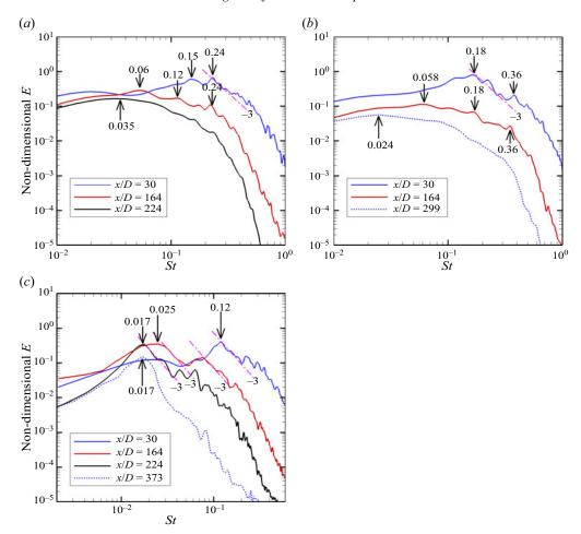
Figure 9. Non-dimensional power spectra of spanwise velocity fluctuations calculated at a point situated close to the TR = 0.5 isocontour and the free surface (z/D = 0.85). (a) Case DS; (b) case DF; (c) case NDD. The straight lines show the presence of a -3 subrange. The arrows point toward peak frequencies in the velocity spectra.
