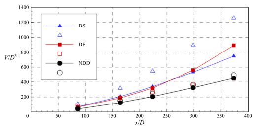
Figure 12. Non-dimensional volume of well-mixed fluid,  $V/D^3$ . The solid symbols are results calculated based on mixing occurring inside the whole domain  $(0 \le z/D \le 1)$ . The hollow symbols are results calculated based on mixing occurring near the free surface  $(0.85 \le z/D \le 1)$ .
