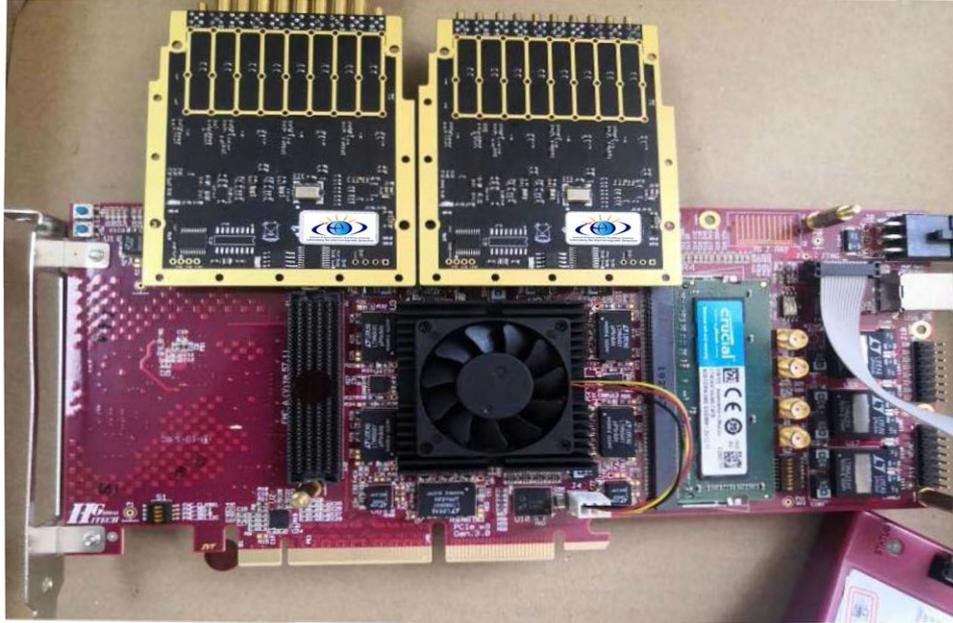
**Figure 4.** Digital Receiver Physical Diagram. The FPGA board is an HTG-830, and more information on the <http://www.hitechglobal.com/Boards/Virtex-UltraScale-FPGA.htm>.
