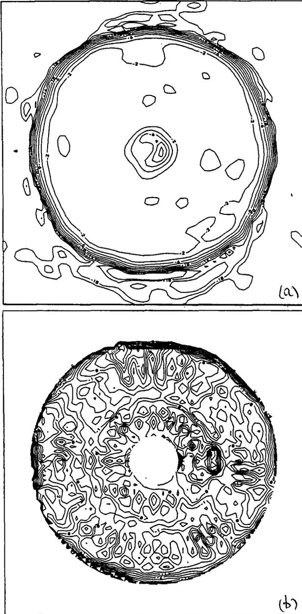
**Fig. 2.** a) Aperture illumination function of a 38-foot antenna with a monopod cassegrain feed. Contour interval is 2 dB. The lowest contour is -20 dB with respect to the maximum power in the aperture. b) Contour map of surface errors for the 38-foot antenna. Contour interval is 0.5 mm.
