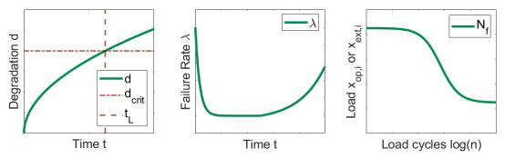
Figure 3. Degradation (left), failure rate (middle) and load cycles (right) as basic model approaches for lifetime prognosis
