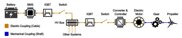
Figure 1. Simplified topology of an electric aircraft powertrain (according to Stückl (2016))
