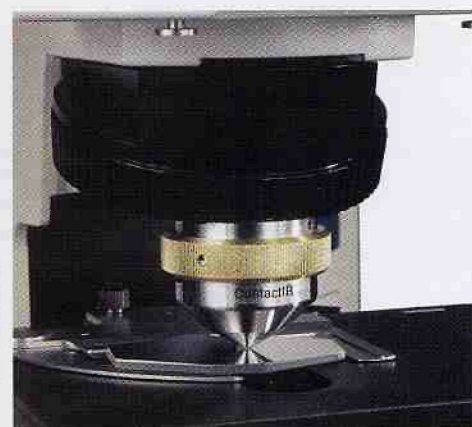
Figure 2 – Schematic of diamond internal reflection objective for micro-ATR spectral data collection. The red area represents the infrared beam path through the objective. The beam from the interferometer enters on one side and reflects from the diamond-sample interface, returning to the detector. The
