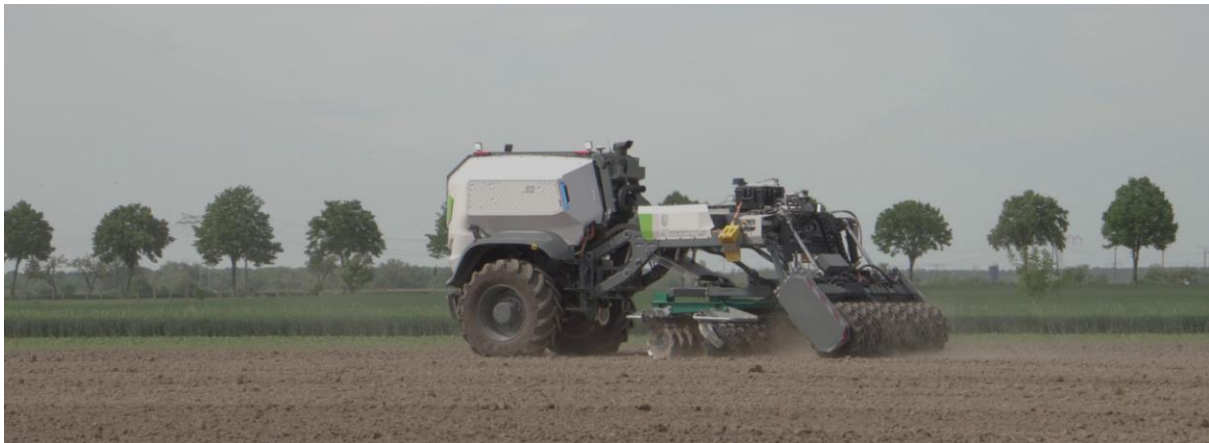
Figure 1: The functional prototype of the Feldschwarm demonstrating automated operation in a tillage mission.
