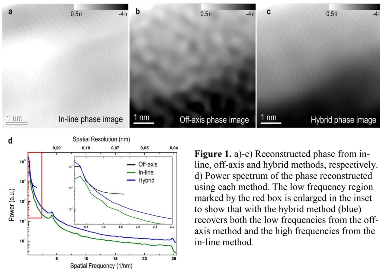
**Figure 1.** a)-c) Reconstructed phase from in-line, off-axis and hybrid methods, respectively. d) Power spectrum of the phase reconstructed using each method. The low frequency region marked by the red box is enlarged in the inset to show that with the hybrid method (blue) recovers both the low frequencies from the off-axis method and the high frequencies from the in-line method.
