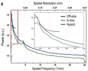
**Figure 1.** a)-c) Reconstructed phase from inline, off-axis and hybrid methods, respectively. d) Power spectrum of the phase reconstructed using each method. The low frequency region marked by the red box is enlarged in the inset to show that with the hybrid method (blue) recovers both the low frequencies from the offaxis method and the high frequencies from the in-line method.
