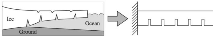
**Fig. 1.** To assess how elastic-flexural waves propagate across a crevasse-ridden ice shelf (left), we analyze the normal modes of a model ice shelf (right).
