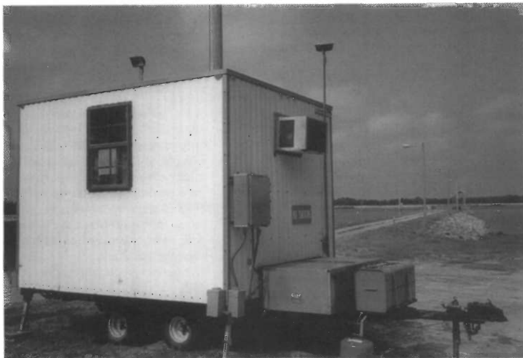
Fig. 5. Trailer housing for FDTAS field unit
