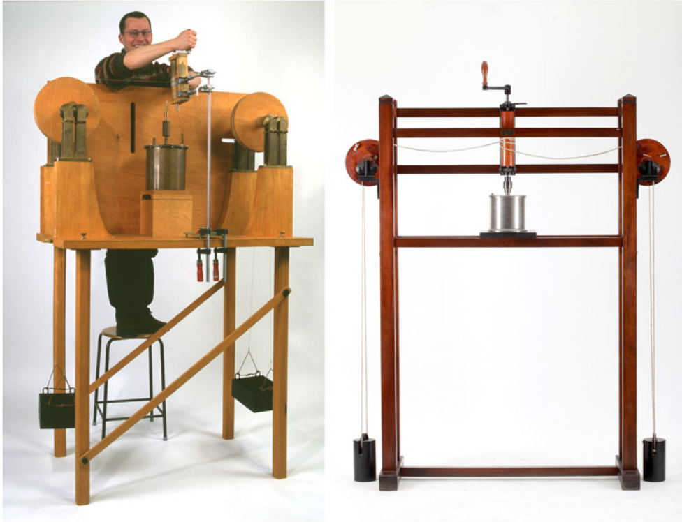
Figure 2. Left: reconstruction of the paddle wheel used in the analysis with the replication method, with permission of the Carl von Ossietzky Universität Oldenburg. Right: teaching version of the paddle wheel apparatus from the company of Max Kohl, with permission of the Fondazione Scienza e Tecnica, Florence.
