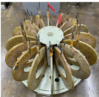
FIGURE 19. (a) The 12 completed PM holder subsegments. Each column is a triplet that makes one quadrant. Y is on the left and X is on the right. (b) The 16 planar, circular TF coils are positioned inside the water-jet cut support structure. (c) The glass VV is joined by 3D-printed low-thickness VV couplers. Glass ports were hot welded to the torus. The PM quadrants accommodate up to three ports each. Seven are installed at present on the north, west and south quadrants.
