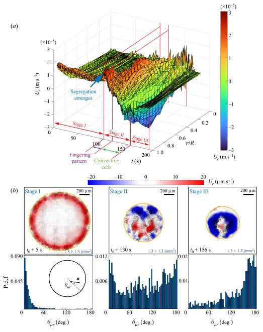
Figure 3. Results from micro-particle image velocimetry ( $\mu$ PIV) in an evaporating 1,2-hexanediol–water binary droplet. The flow field near the substrate is revealed. (*a*) A 3-D map showing the temporal evolution of the radial velocity averaged in azimuthal angle along the radial position. (*b*) The probability distribution function (p.d.f.) of the azimuthal angle of the flow velocity versus the radial direction at three different life stages.
