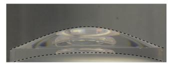
**Figure 5.** A comparison of experimental results (image within the liquid container) to our theoretical predictions (dashed lines), for  $\Delta \rho = -6.5 \text{ kg/m}^3$ , D = 87.2 mm,  $V_{lens} = 48 \text{ ml}$  and  $\gamma = 0.02 \text{ N/m}$ , yielding good agreement with no fitting parameters.
