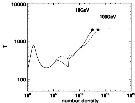
**Figure 2.** Temperature (in degrees K) as a function of hydrogen density (in  $\text{cm}^{-3}$ ) for the first protostars, with DM annihilation included, for two different DM particle masses (10 GeV and 100 GeV). Moving to the right in the figure corresponds to moving forward in time. Once the “dots” are reached, DM annihilation wins over H<sub>2</sub> cooling, and a Dark Star is created.
