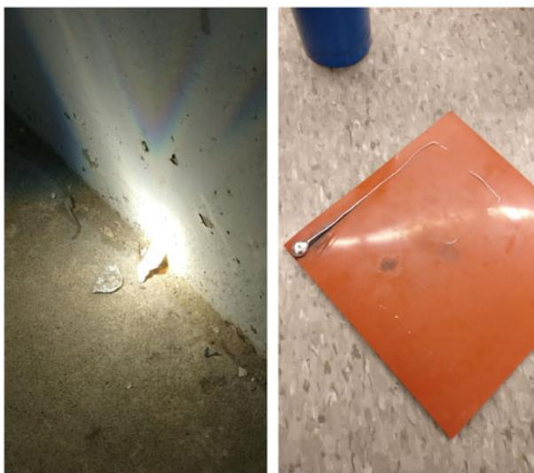
**Fig. 1.** (a) Fresnel lens melting of aluminium alloy; (b) molten aluminium directly on silicone plastic.
