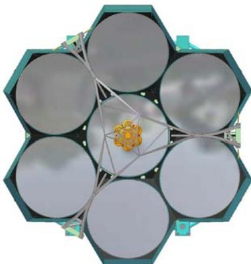
**Figure 3.** This top view of the telescope shows the small foot print of the secondary supports and shape of the GMT pupil. This secondary configuration results in excellent thermal performance and a PSF free of diffraction spikes associated with conventional secondary supports.
