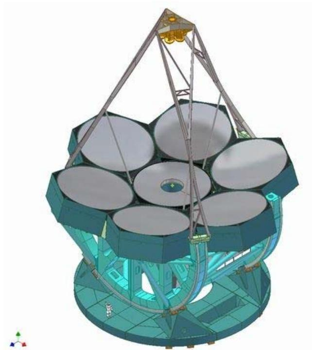
**Figure 1.** A rendering of the Giant Magellan Telescope. The mount is of the altitude-azimuth variety and uses two large C-rings to support the primary mirror assembly. The telescope moves in azimuth by rotating on hydrostatic bearings riding on a ring beam. The telescope stands 36m high and is 25.5m wide. Instruments are located behind the central primary mirror segment.
