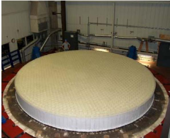
**Figure 7.** The GMT prototype primary mirror segment on the hearth at the Steward Observatory Mirror Laboratory. The mirror is cast in a rotating oven and while it is cast with a circularly symmetric top face, an asymmetric distribution of mold cores ensures that the final off-axis mirror will have a uniform thickness top sheet. The prototype mirror is scheduled for completion in early 2008.
