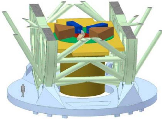
**Figure 4.** This cut-away view of the telescope highlights the upper instrument platform and shows the large straight Gregorian focus instrument bay. The upper platform will house a number of instruments available for rapid response to changing conditions or time-critical astronomical events. The 8.9m diameter disk rotates to provide field derotation for all of the upper platform instruments.
