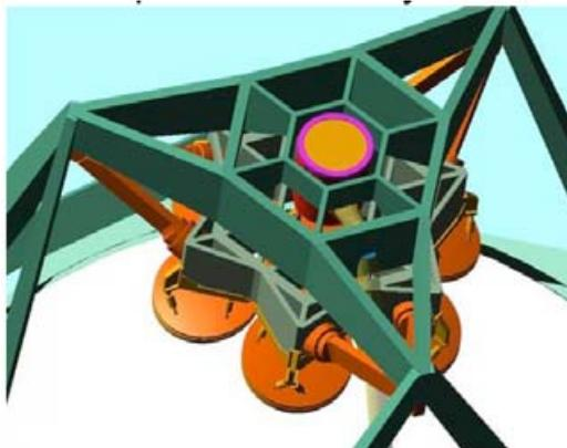
**Figure 2.** The GMT secondary mirror is composed of seven 1.06m diameter segments, each of which addresses one of the primary mirror segments. The baseline design calls for thin-shell adaptive segments, although conventional light-weighted fast-steering segments might be used for commissioning. The secondary is concave, producing an  $f/8.0$  aplanatic Gregorian final focus.
