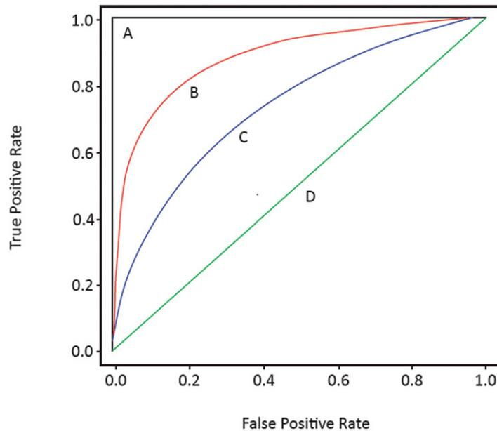
**FIGURE 2.** (A–D) Contrasting Receiver Operating Characteristic (ROC) curves (after Sing et al. 2005). A perfect test (A) has an area under the ROC curve of 1.0. The diagonal line (D) from (0, 0) to (1, 1) has an area under the ROC curve of 0.5.
