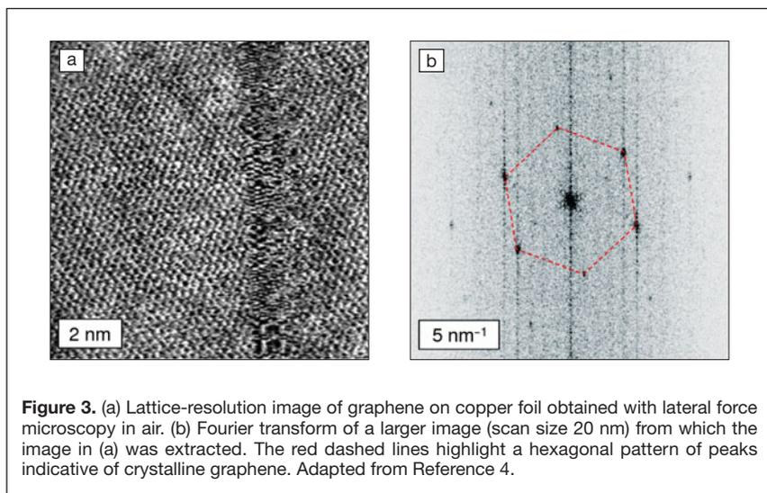
**Figure 3.** (a) Lattice-resolution image of graphene on copper foil obtained with lateral force microscopy in air. (b) Fourier transform of a larger image (scan size 20 nm) from which the image in (a) was extracted. The red dashed lines highlight a hexagonal pattern of peaks indicative of crystalline graphene. Adapted from Reference 4.
