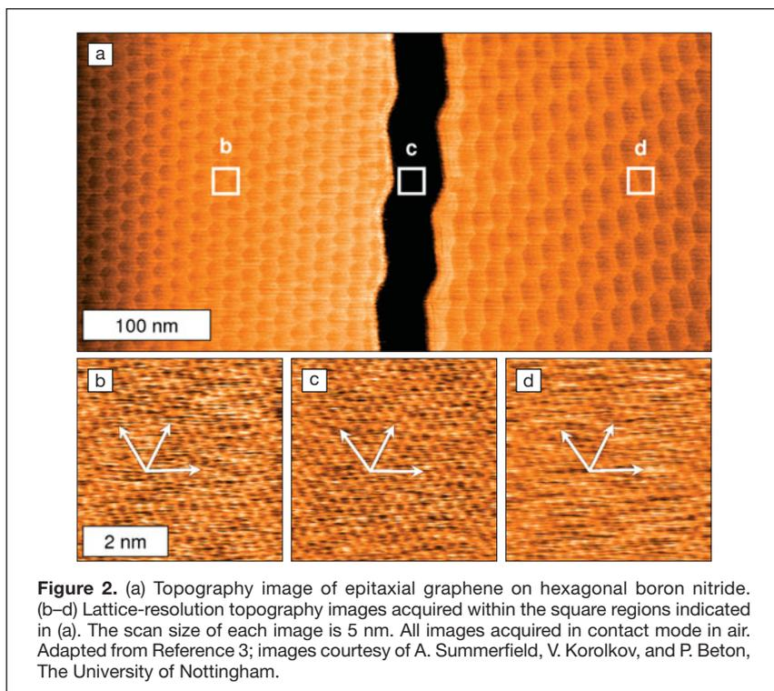
**Figure 2.** (a) Topography image of epitaxial graphene on hexagonal boron nitride. (b–d) Lattice-resolution topography images acquired within the square regions indicated in (a). The scan size of each image is 5 nm. All images acquired in contact mode in air. Adapted from Reference 3; images courtesy of A. Summerfield, V. Korolkov, and P. Beton, The University of Nottingham.
