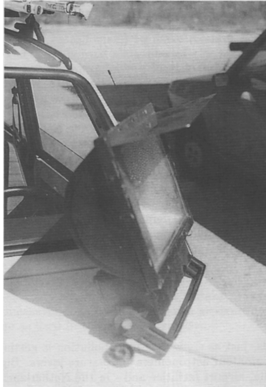
Figure 4. Modification of a symmetric beam with a simple metal screen. No more light in the sky! Cost: US$2 each.
