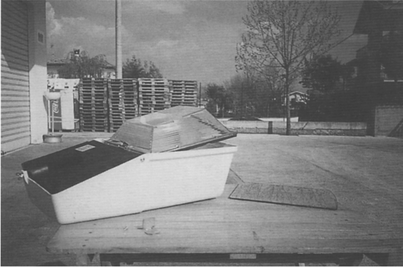
Figure 1. Modification of street lighting fixtures with a flat tempered glass to give more transmission of light onto the road, with drastic reduction of glare and light-pollution. Cost: US$5 each.
