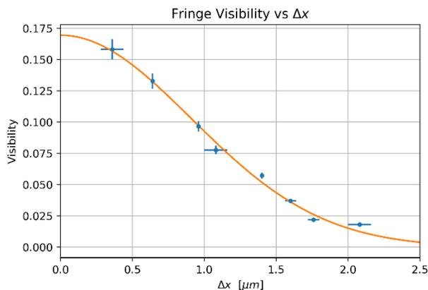
**Figure 2.** Fringe visibility over a 2.5  $\mu\text{m}$  range of diffraction probe separation. The data has been fit to a Gaussian curve in order to measure the coherence width of the electron source in this TEM. We find that the coherence width is  $1.81 \pm 0.04 \mu\text{m}$ .
