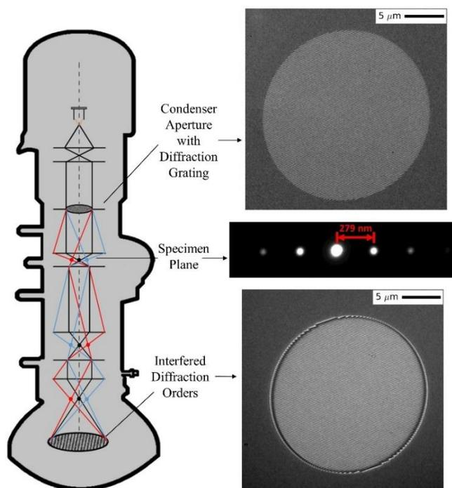
**Figure 1.** Experimental setup. The diffraction grating is placed in the condenser aperture of the TEM. Diffraction probes are visible in the specimen plane and are interfered in the image plane to produce interference fringes.
