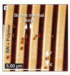
Figure 1. (a) Typical atomic force microscope topography image shows a low-dielectric polymer coating covering trenches in a model microelectronics trench structure. (b) The corresponding scanning near-field ultrasound holography phase image reveals embedded voiding in the polymer coating over the nitride. Reprinted with permission from Science (Oct. 7, 2005) p. 89. ©2005 **AAAS**.
