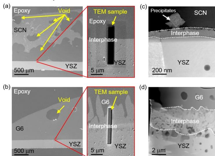
**Figure 1.** SEM images of (a) SCN-1/8YSZ and (b) G6/8YSZ after 40,000 hours exposure to air at 800 °C. High-magnification SEM images (right) show location of TEM sample lift-out. STEM high-angle annular dark-field (HAADF) images of (c) ~ 200 nm thick SCN-1/8YSZ interphase and (d) ~ 2 μm thick G6/8YSZ interphase.
