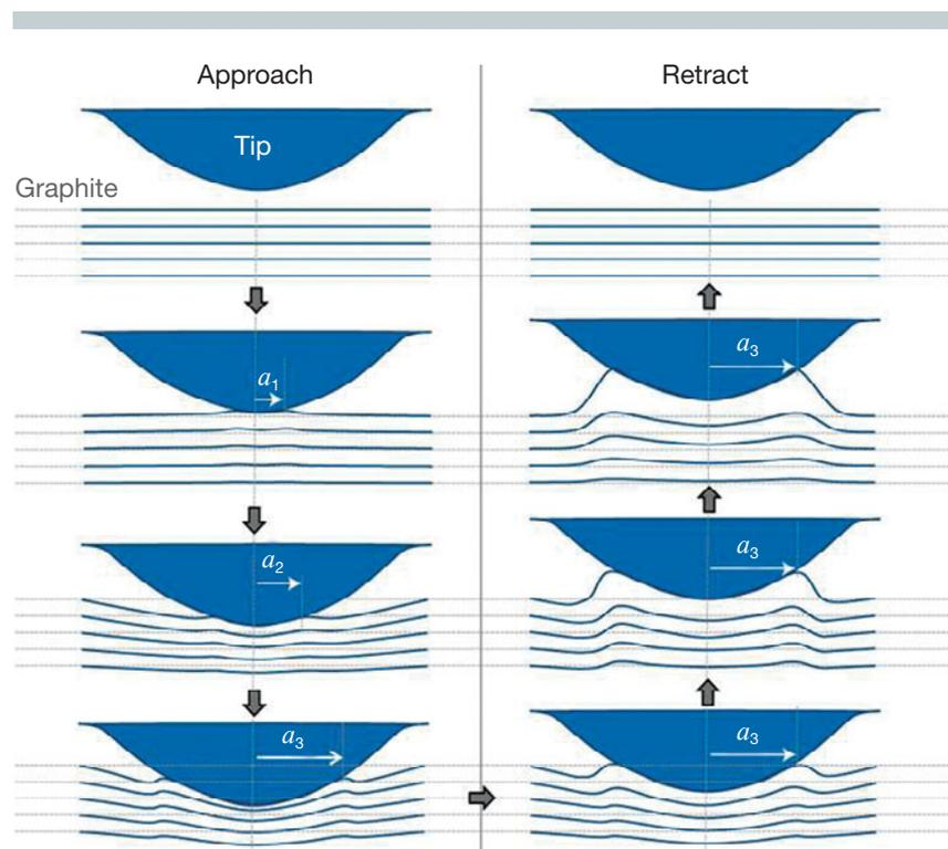
Schematic representation of approach-retract hysteresis in the deformation of several surface and subsurface layers of graphite. Reproduced with permission from *Nature Mater.* **11** (2012), DOI: 10.1038/NMAT3452; p. 1032. © 2012 Macmillan Publishers Ltd.
