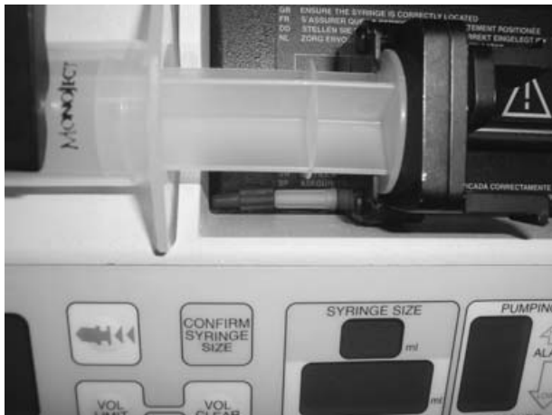
Figure 1. Two caps of the extension set obstructing the syringe driver's mechanism.
