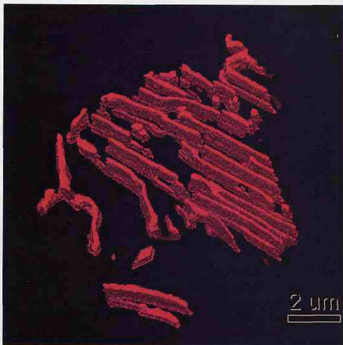
Figure 4: A volume reconstruction of a Cu-In lamellar colony reconstructed using secondary electron images and shape base interpolation. The red structures shown in this reconstruction correspond to the lamellae shown in Figure 3.
